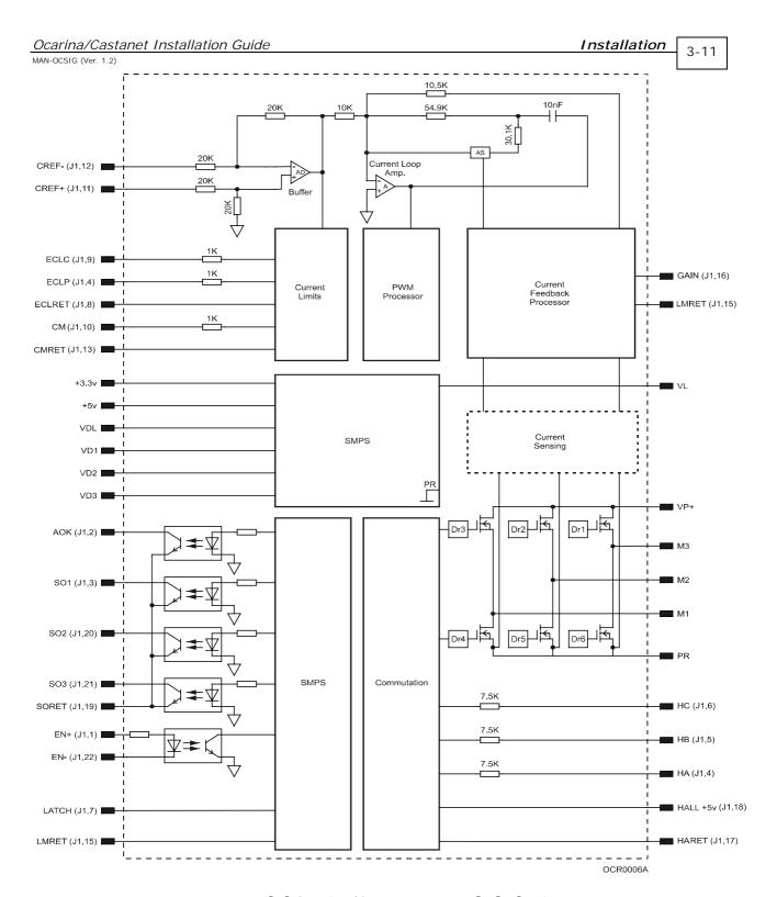
Figure 3-4: Detailed Ocarina/Castanet Internal Block Diagram
